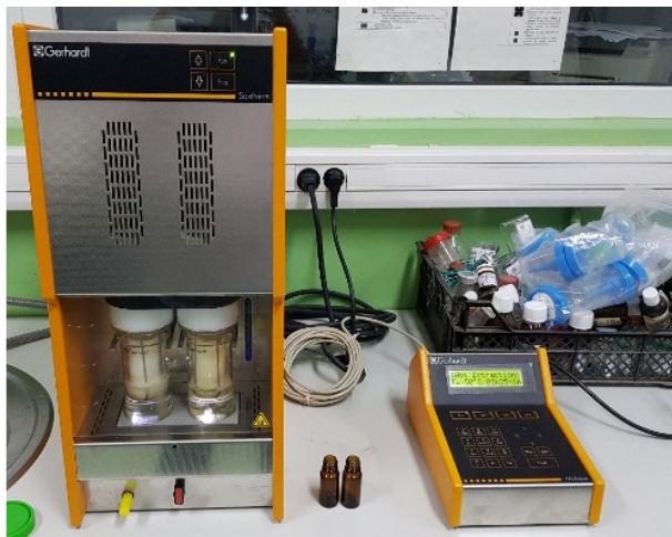
Figure 4. Oil extraction using Gerhardt Soxhlet apparatus
