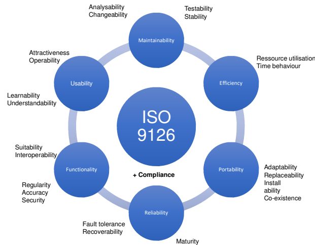
Fig. 3: Model ISO 9126 (adapted from ISO 9126)
